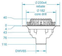
Inlet Size - 100 mm Outlet Size - 65 mm Flow Rate - Contact RL Code - 3100.176
