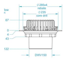
Inlet Size - 150 mm Outlet Size - 150 mm Flow Rate - 1800 l/min Code - 3100.305
