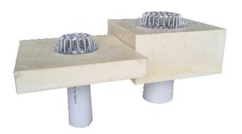
The area surrounding the drain in a box gutter is frequently overlooked or haphazardly filled with insulation off-cuts. This can result in a sub-par installation of the roof drain and diminished R-Values in that specific region due to thermal bridging.
