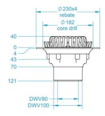
Inlet Size - 100 mm Outlet Size - 80 mm/100 Flow Rate - 500 - 1000 l/min Code - 3100.205
